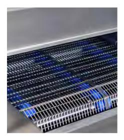
Liquid nitrogen and CO2 deliver the ultimate in cryogenic freezing power by minimizing any aroma, flavor and dehydration losses to the food product. Because these cryogenic gases are inert, they also provide a protective atmosphere inside the freezing zone which prevents any oxidation of the food. As a result, the quality attributes of cryogenically-frozen food products are far superior to those same products frozen in a mechanical system.
