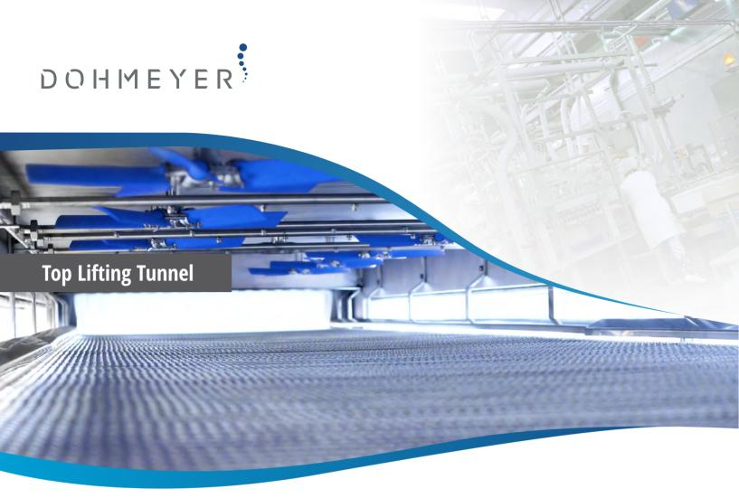
Dohmeyer's in-line cryogenic freezing Tunnels are commonly used to freeze all kinds of foods ranging from small diced products to larger whole muscle meat or packaged products.
